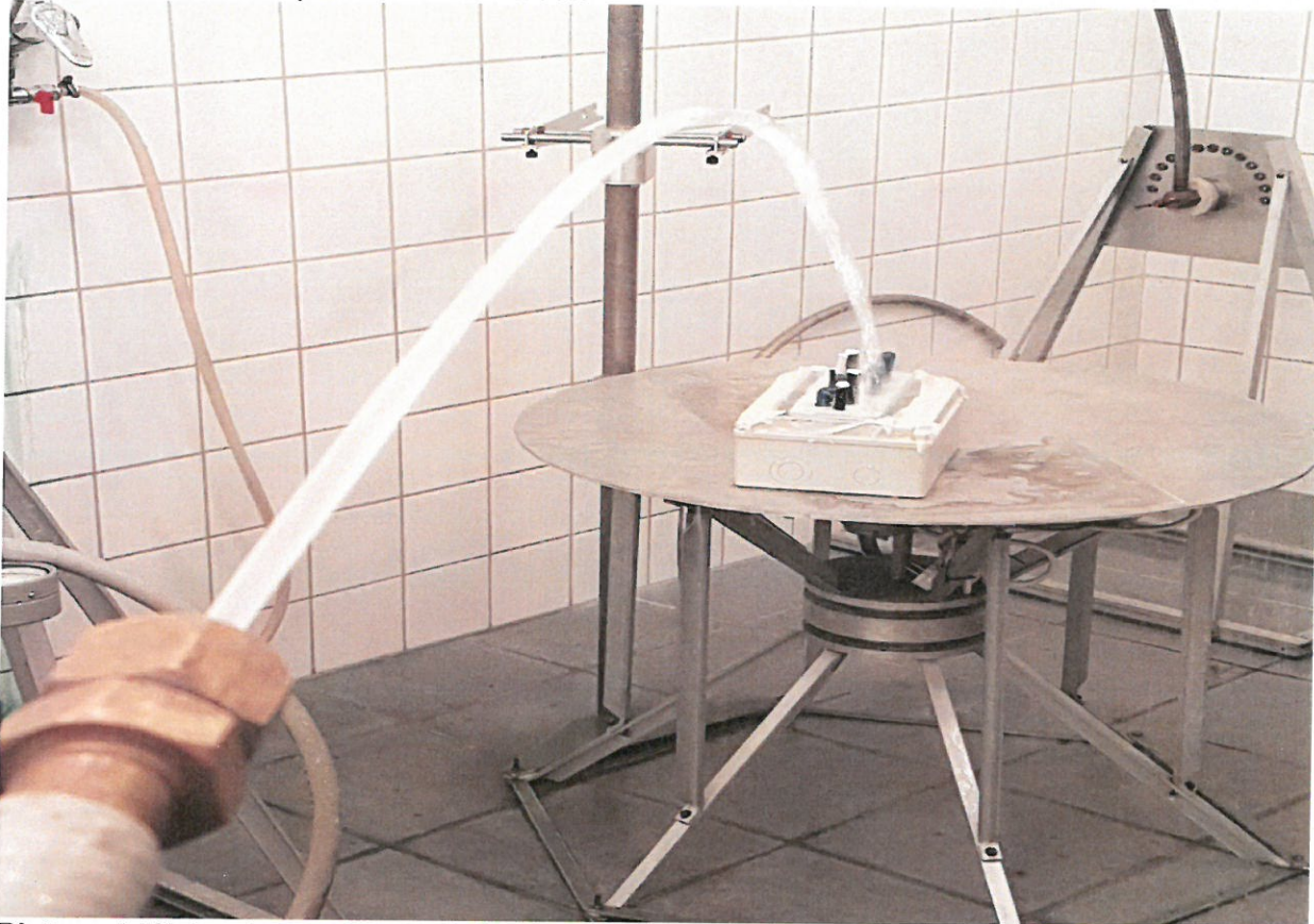
Picture 4. Water does not enter through the flange and its confirmation
