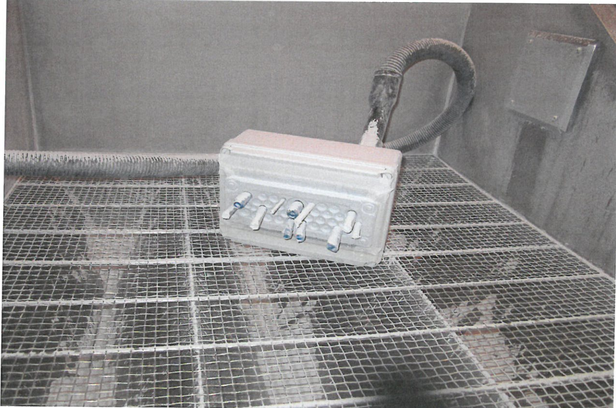
Picture 6. Samples HTKC-36 after test IP6X
